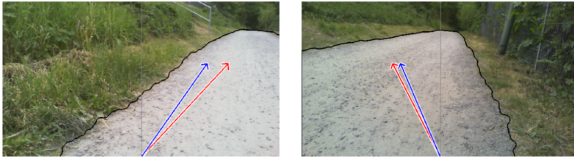
Fig. 4. Comparison of the results of the original algorithm (red) and the algorithm with our modifications (blue). The generated control signals differ slightly, but still deliver safe results to control the Ceres UGV.
